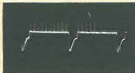
Well defined back porch on horizontal sync pulse permits accurately setting color killer and almost eliminates need to adjust brightness and contrast.
